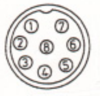
Figure 6-3 ID Numbers of Pins in I/O Data Receptacle Viewed from Plug (Cable) Side
