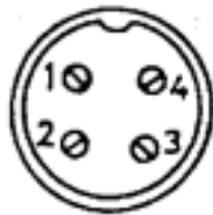
Figure 6-4 ID Numbers of Pins in Water Temperature Sensor Receptacle Viewed from Plug (Cable) Side
